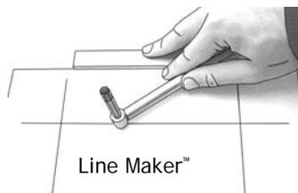
5. Align the rule on the pencil line so the line is just visible, then attach the #201 cutting head to the rule - see fig. 2. The Mat Master™ #201 head will cut accurately on the line everytime.
