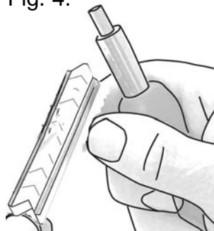
Place V-Nail around the magnetic tip of the Ezy-Framer.
