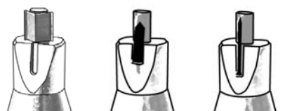
Magnet holds V-Nail Flexipoint Slot Backing Nail Slot
