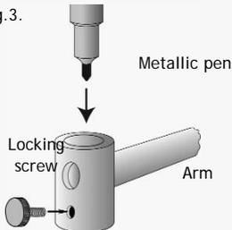
The Line Maker™ is a quick and easy way to mark a mat ready for bevel cutting.
