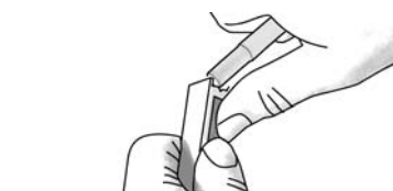
Fig 6. Pull the WedgeMate upwards to pry off one v-nail from the end of the cartridge.
